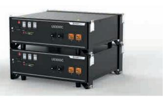
The storage modules comprise a lithium iron phosphate (LiFePo4) accumulator and an integrated battery management system (BMS) which constantly monitors the status of individual cells and these also provide protection against excessive levels of charge, voltage and temperature. This is how the BMS prevents an accumulator from failing prematurely as a result of ambient factors or operator error.
